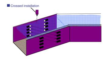
For simple open channel monitoring problem channel bottom or side mounted Doppler effect based devices offer a cost effective solution.
